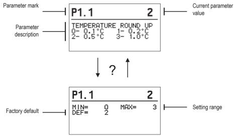
The setting is changed by pressing the button  $\checkmark$ .
