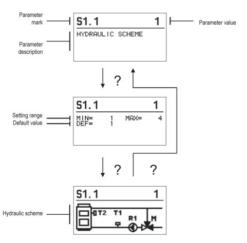
The setting is changed by pressing the button  $\checkmark$ . Because the parameters are factory locked, a new screen appears. Here you have to enter the unlock code.
