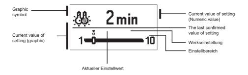
You change settings by pressing buttons – and + and confirm by pressing button  $\checkmark$  .
