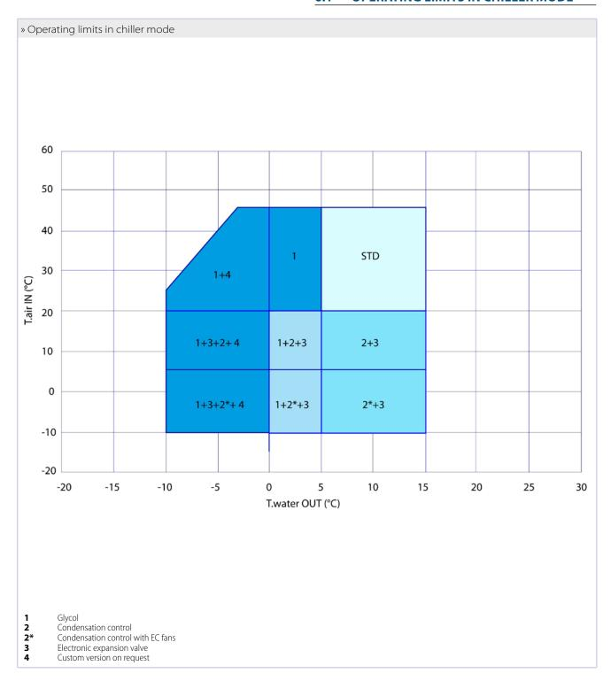
To operate with outdoor temperatures below 20  $^{\circ}\text{C}$  and above 5  $^{\circ}\text{C}$  it is essential to employ the (optional) condensation control with phase cutting device.
