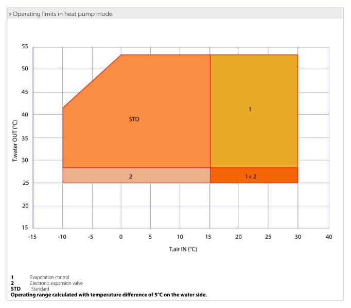
To operate with outdoor air temperatures below 0°C the temperature of the water produced will be reduced to 45°C. It is essential to use the (optional) device to monitor evaporation to detect the outlet water temp. from the condenser with an ambient temperature of the air greater than 20°C. For temp. of produced water between 25°C and 30°C is it compulsory to use an electrical expansion valve.
