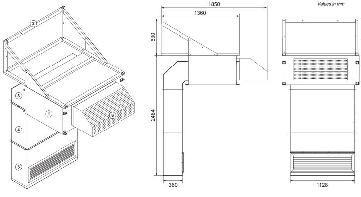
1 DUCT AIR split system internal unit
