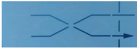
Fig. 34: Free heating o Free cooling attivo / Free heating or Active free cooling
