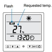
Once the symbol SI stops flashing, there quested temperature will be validated and up to the temperature of the water current (in our example 25 °). Your screen will display:
