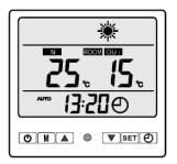
Heating mode Select for the heating mode In this mode, the heat pump will heating the water in your pool.
