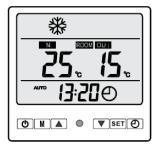
Cooling mode Select 🏶 for the cooling mode In this mode, the heat pump will cooling the water in your pool.
