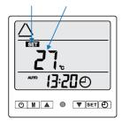
Once the symbol **San** stops flashing, the requested temperature will be validated and up to the temperature of the water current (in our example 25 °). Your screen will display: Current ambient temp.
