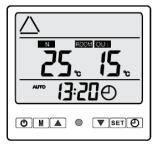
Automatic mode (hot, cold) Select for the Auto mode In this mode, the heat pump will automatically change to heating or cooling your pool (depending on the actual tempera ture) to reach the desired temperature. No electric heating.
